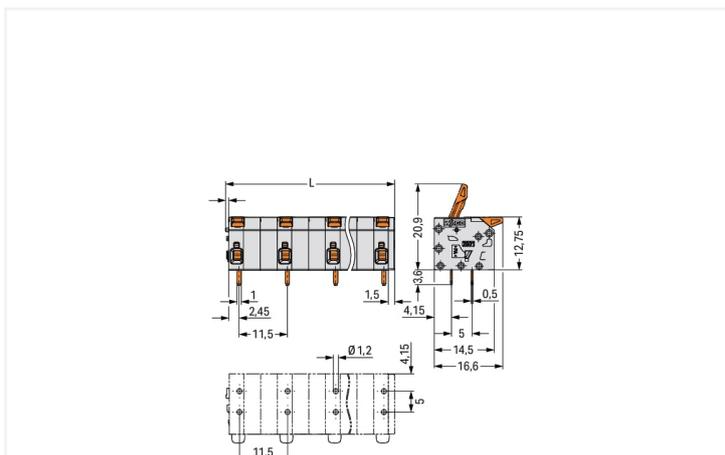
$L = (\text{pole no.} - 1) \times \text{pin spacing} + 5 \text{ mm}$
