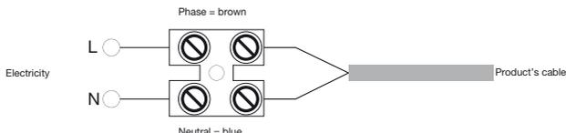
In humid rooms, bathrooms or kitchens, this connection block must be installed at least 25 cm from the floor. The electrical connection must also include the use of a 2-pole switch with a contact opening distance of at least 3 mm.
