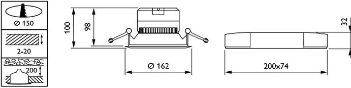
DN140B LED10S/840 PSD-E WR IP54
