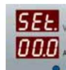
After 4 seconds the pages with configuration parameters start to be displayed; one page every 4 seconds showing the actual selected value. If it is necessary to see the values without any modification don't touch nothing until the automatic end of the showed pages.
