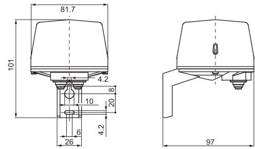
**3 - DESCRIPTION**
