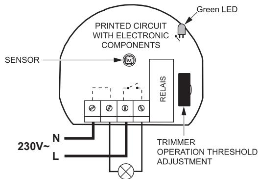
**6 - OPERATION THRESHOLD ADJUSTMENT (LUX)**
