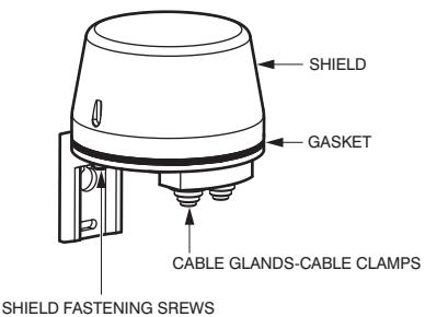
**4 - INSTALLATION PROCEDURE****Installing the twilight switch**
