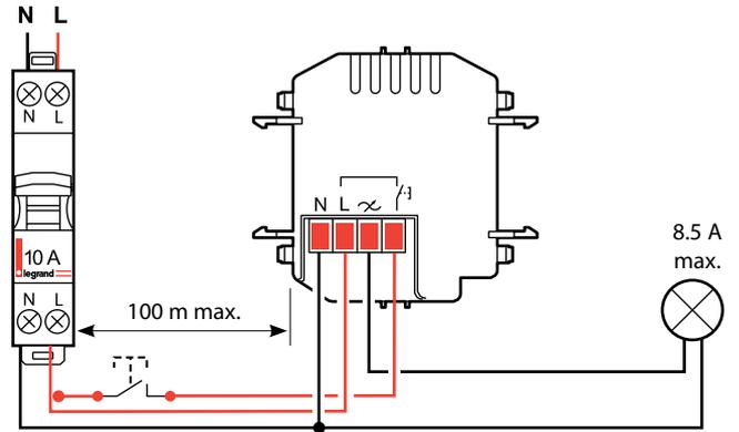
■ **4.2 Wiring without auxiliary control: Auto on/Auto off**
