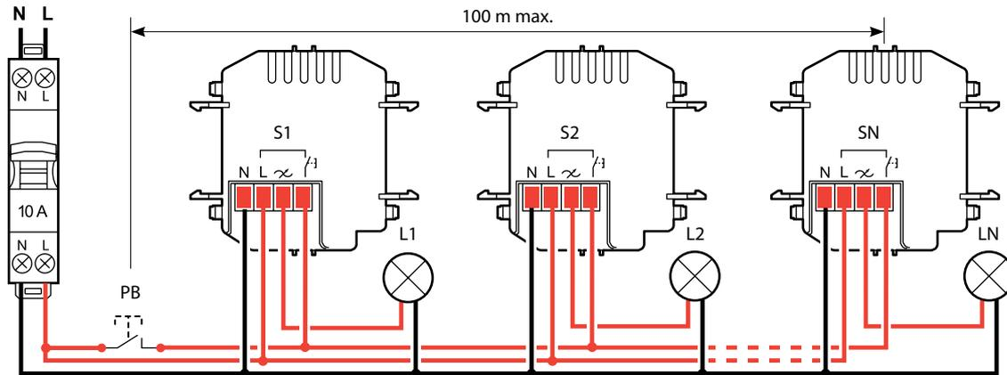
■ 4.4 Wiring for a single load connected in parallel
