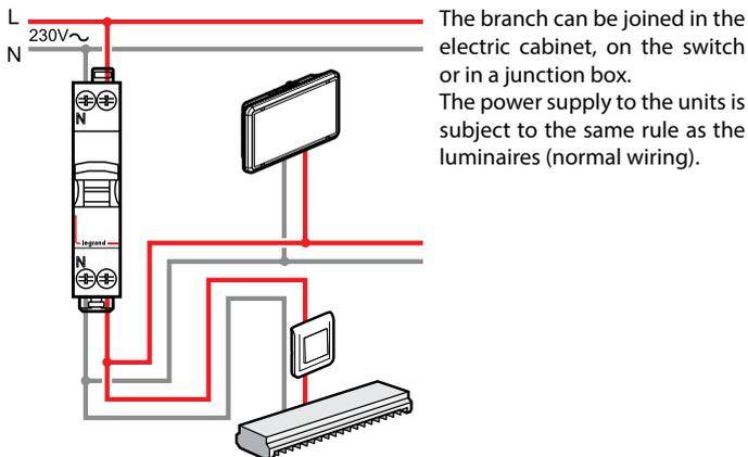
The branch can be joined in the electric cabinet, on the switch or in a junction box. The power supply to the units is subject to the same rule as the luminaires (normal wiring).
