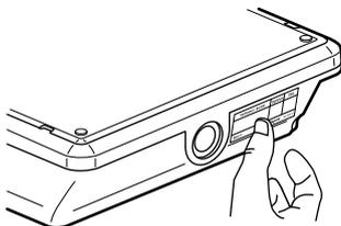
This maintenance label (Cat. No. 0 609 00) must be attached to each lighting unit in a position where it can be seen, and marked with the date on which the unit was commissioned.
