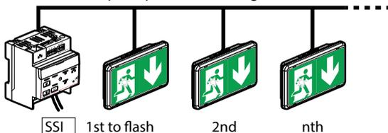
This parameter setting must be done with configuration tool Cat. No. 0 882 40 and the CloseUp app. This action can assign a number that indicates the unit position in the queue.
