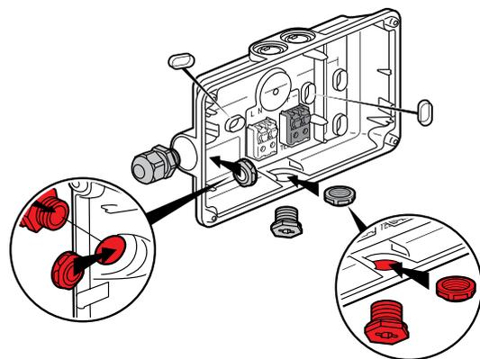
**Caution:** Ensure the nut is fitted the right way round, as shown above. As soon as installation is complete, attach a maintenance label Cat. No. 0 609 00 and write the commissioning date on it (see 5.1). Attach the adhesive separable signalling label (supplied with the unit).
