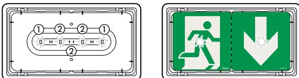
Both outdoor emergency LEDs come on (45 lm) for emergency lighting unit function ①
