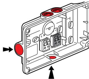
The product is shipped with 2 drilled holes for feeding through the cables, one of which (depending on the incoming cable) should be fitted with the cable gland and the other with the plug.
