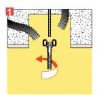
The independent duct is screwed onto the threaded rod sealed in the
