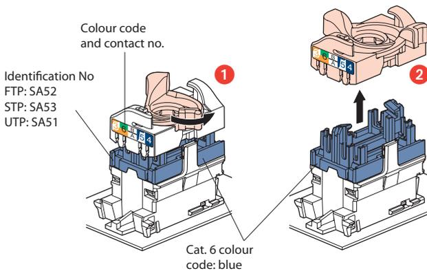
This system makes it easy to spread pairs before fitting them onto the connector.
