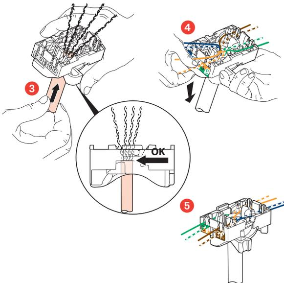
Spreading the cables ensures that a pair-breakage distance of 13 mm is kept between each pair.
