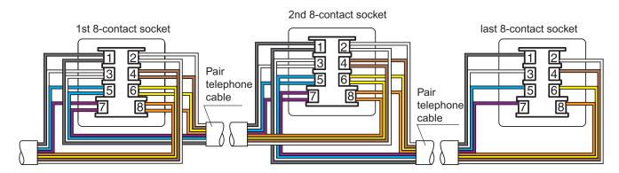
Connect the sockets in parallel: all wires must be connected. Use France Telecom approved cable, 4 pairs,  $\varnothing$  0.6 mm, type 278-4.6. Follow contact numbers and wire colours.
