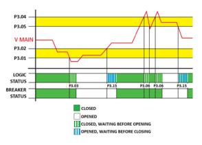
Example of variation of the main line voltage within the minimum and maximum thresholds and relative hysteresis, with indication of the presence / absence delay times. The example considers the secondary line voltage absent with its circuit breaker open, hence the changeover times are not shown. The BREAKER STATUS bar represents the required status of the main line switch, while the LOGIC STATUS bar represents actual logic status of line controller.
