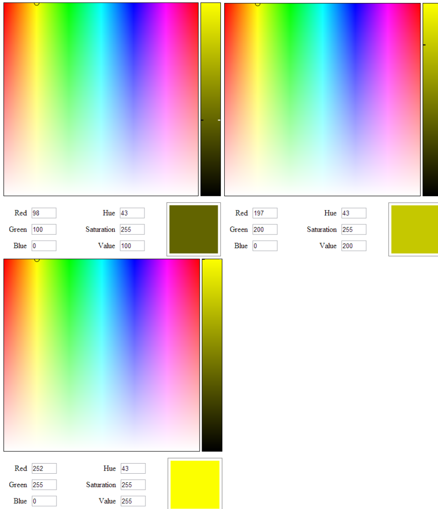
Fig. 3.5: Example of colour regulation based on the HSV system (Tone, Saturation and Brilliancy)
