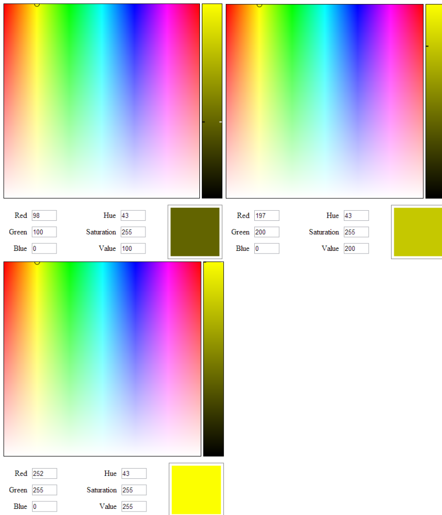
Fig. 4.3: Example of colour regulation based on the HSV system (Tone, Saturation and Brilliancy)
