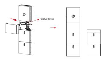
If you connect more than 2 battery modules to the system, please install only additional batteries 4, 6 and 8 on the side of the system.
