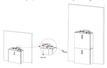
**Step 5** To assemble the second (and all other) battery, repeat steps 2 and 3 respectively.
