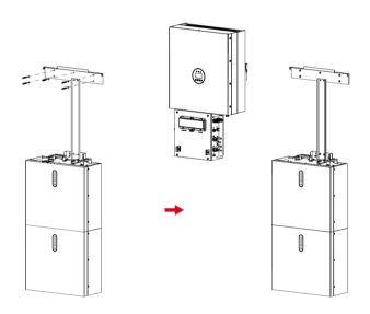
**Step 1** Hang the inverter onto the mounting panels, adjust the entire system and ensure that the battery and the inverter have been securely hung onto the panels and brackets.
