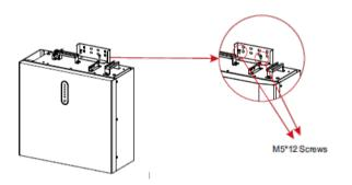
**Step 3** Position the battery parallel to the wall and use a Φ8mm drill to drill holes at a depth of about 70mm in the wall for subsequent fixation of the mounting plates.
