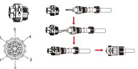
**Step 2** Install the waterproof component and screw on the waterproof sheath nut
