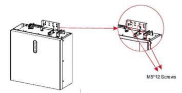
Step 3 Position the battery parallel to the wall and use a Φ8mm drill to dril holes at a depth of about 70mm in the wall for subsequent fixation of the mounting plates.
