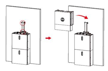
Step 1 Hang the inverter onto the mounting panels, adjust the entire system and ensure that the battery and the inverter have been securely hung onto the panels and brackets.
