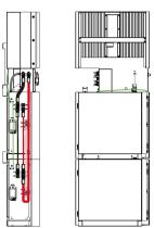
**Step 5** Close the battery covers and connect the PV-MC4 connectors to the system (connect ion on both sides).
