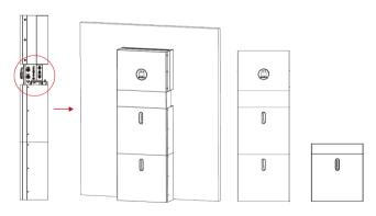
If you connect more than 2 battery modules to the system, please only install the additional batteries. If you connect more than 2 battery modules to the system, please only install the additional batteries 3, 4 &5 on the side of the system. You can connect to 5 batteries, 3 each mounted on top of each other, to the XST Home Inverter.
