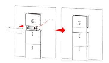
Step 8 Close the lid and tighten the screw. The installation is now complete.
