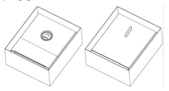
**Step 2** Assemble the battery mounting panel on the battery.
