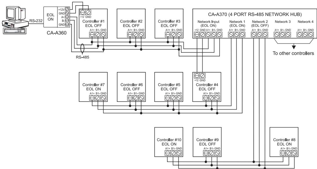
Note: The distance between the first and last device in each network should not exceed 3000 feet (1.2km).
