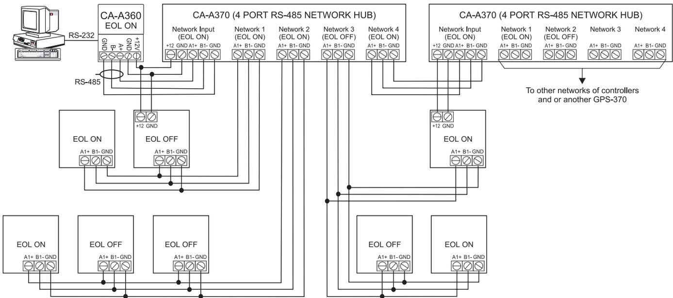
Note: The distance between the first and last device in each network should not exceed 3000 feet (1.2km).
