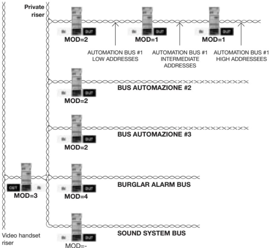
2. With systems without a logical expansion but with a physical expansion, the interfaces toward the Burglar alarm, Sound System and Video door-entry system must be connected to the bus with lower addresses.
