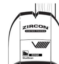
Continue sliding tool. When the centre of stud is located with three bars on the Signal Strength Indicator, some segments of the Target Indication bars, CENTER indication, and SpotLite® Pointer will all illuminate, and the buzzer will sound.
