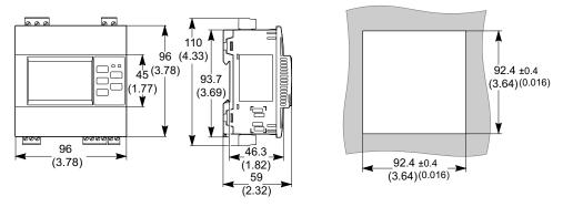
Observe the correct distances between devices for flush-mounting as per the following figure:
