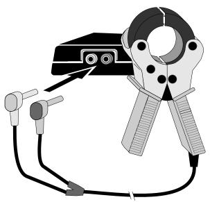
3. Clamp the XPxx and XRM setup to an inject wire near to the device.
