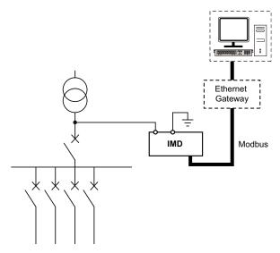
**NOTE:** Using an Ethernet gateway enables you to make use of an existing Ethernet network.
