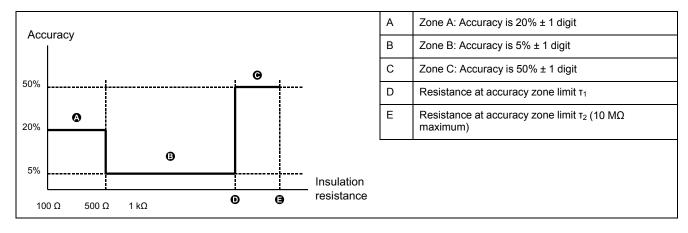
Assuming two significant digits for insulation resistance measurements the accuracy can be calculated.
