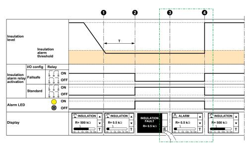
An insulation fault is detected on the system..
