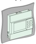
2. Depending on the thickness of the mounting plate, clip the 3 spring clips into the fixing slots on the device as follows:
