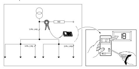
5. Clamp the XPxx and XRM setup on all the channels and record the XRM values on each channel.
