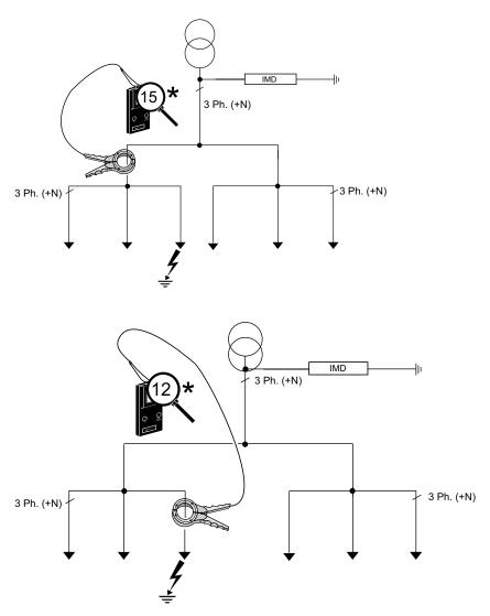
If the recorded value of a channel is nearest to the calibrated value, it indicates an insulation fault in the corresponding channel or the downstream channel (if any).
