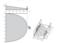
In order to ensure continuous monitoring, e.g. of a long hall, the areas of detection of the individual movement detectors have to intersect.
