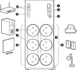
audio/visual receiver to the Master outlet. Connect peripheral devices such as a printer, speakers, or a scanner to the Controlled outlets.
