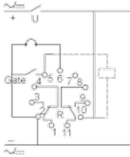
Function L : Asymmetrical Flasher Relay (Starting Pulse Off)
