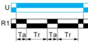
Function Lt: Asymmetrical Flashing Relay (Starting Pulse Off) & with Pause / Summation Control
