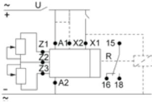
Function L: Asymmetrical Flashing Relay (Starting Pulse Off)
