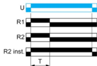
Function Hw: Interval Relay & with Retrigger / Restart Control
