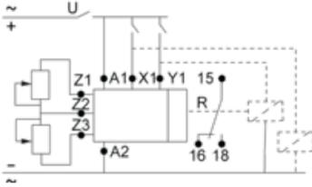
Function Ak: Asymmetrical On-Delay & Off-Delay with Control Signal
