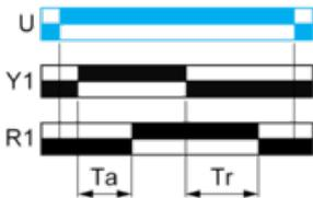
Function Akt: Asymmetrical On-Delay & Off-Delay with Control Signal & with Pause / Summation Control
