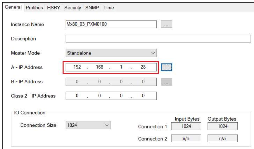
Figure 3.83 – Confirm matching IP address in Configuration Utility
