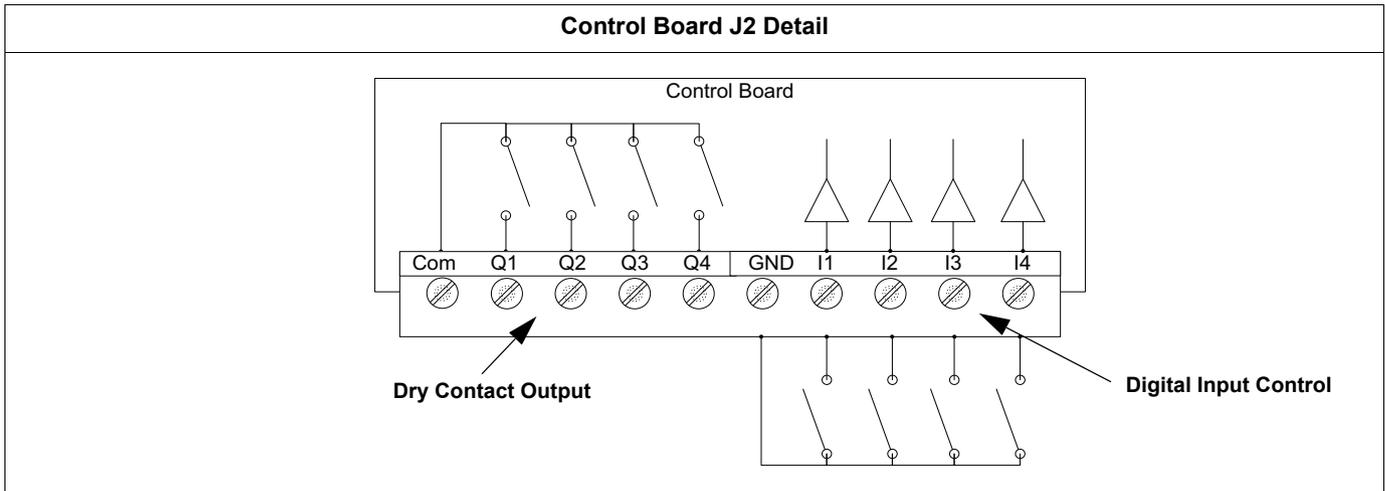
**NOTE:** The control board J2 accepts wire size between 0.2 mm<sup>2</sup> (24 AWG) and 2.5 mm<sup>2</sup> (12 AWG).
