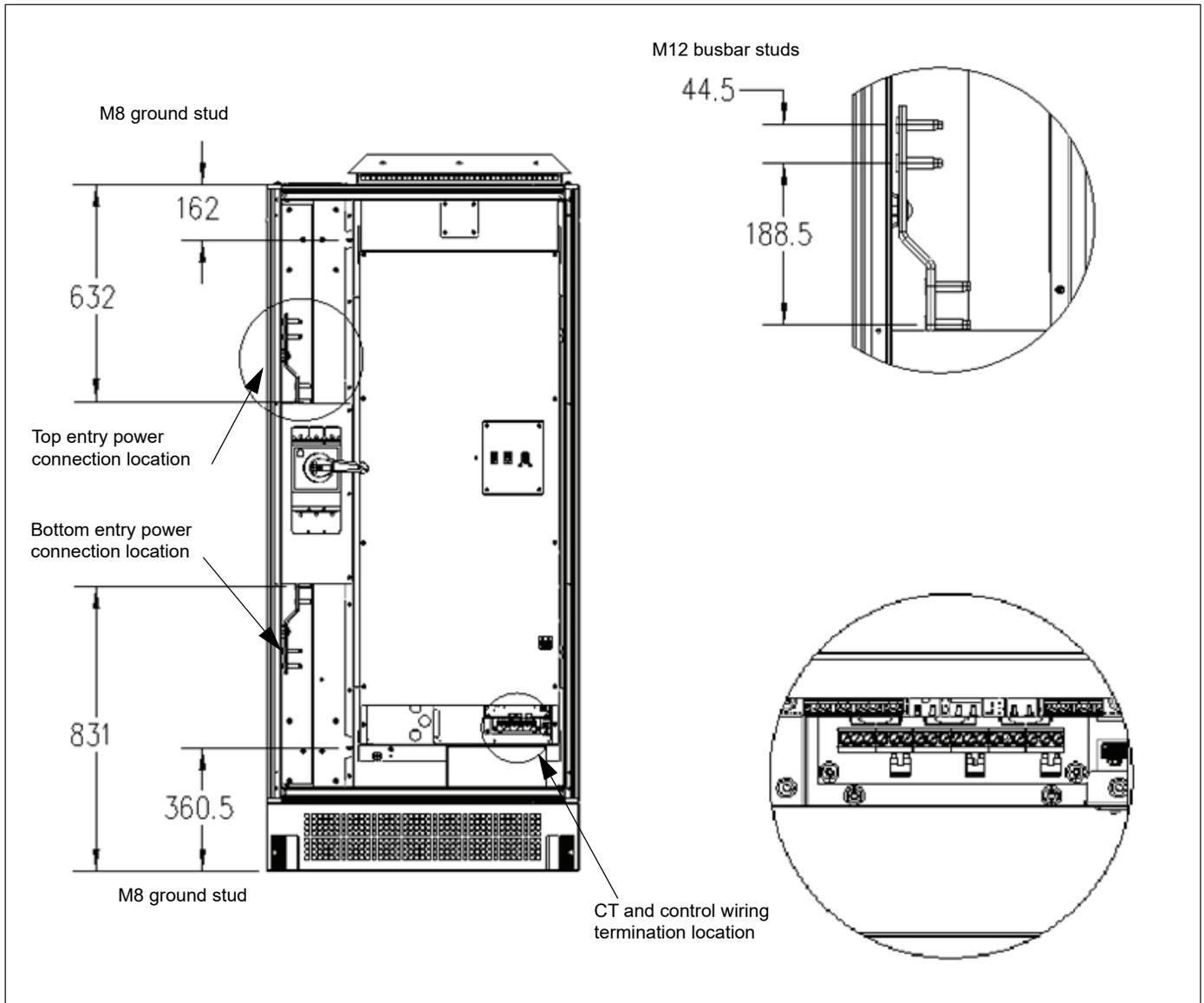
200 A and 300 A UL Type 1 IP20 Enclosure Internal Layout Drawing
