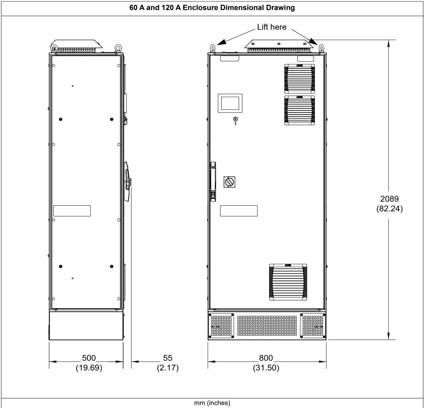
**NOTE:** The diagram is of an IP54 model. The IP31 models do not have air intake vents on the door.
