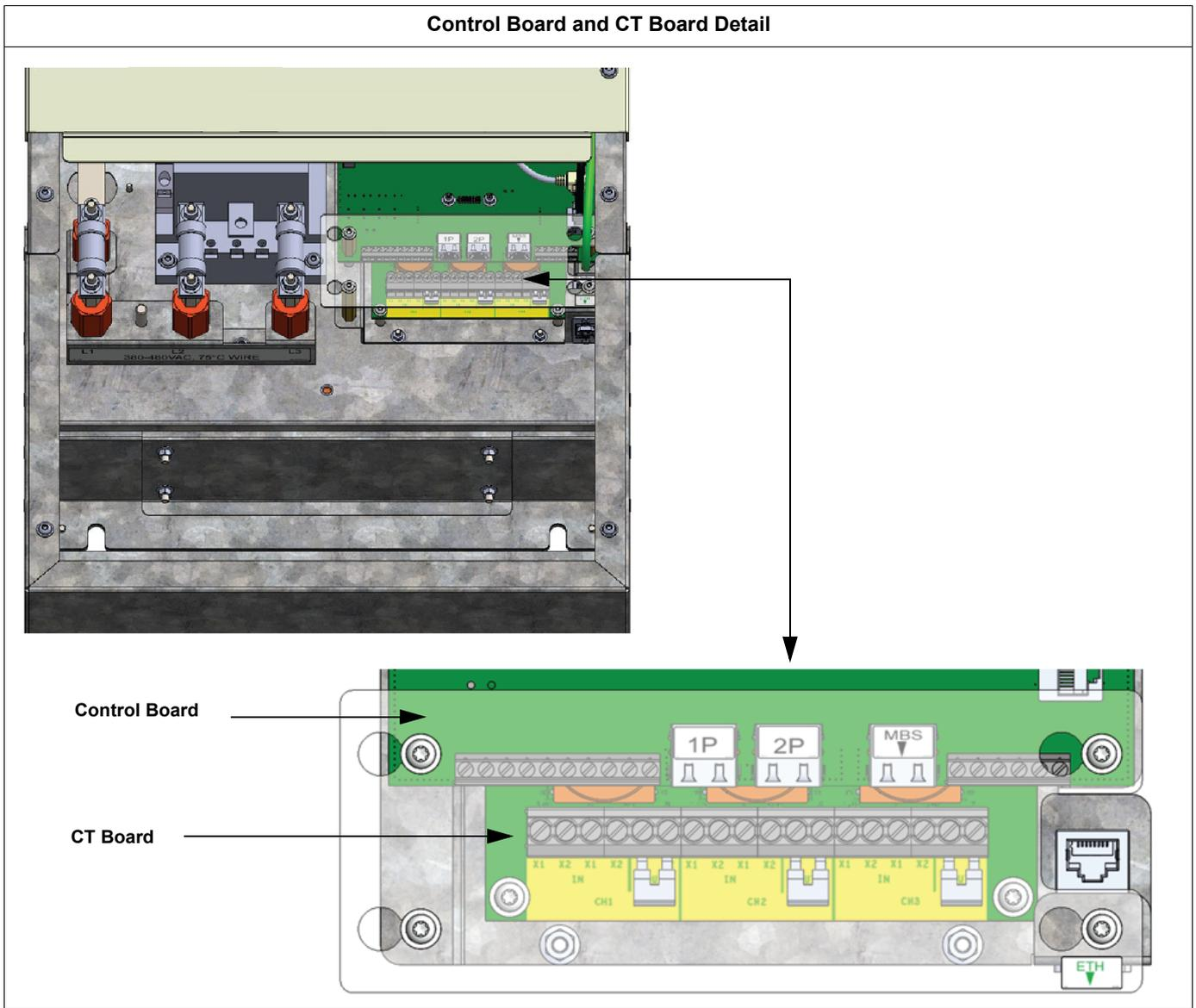
The terminal block on the CT board can accept wire sizes of up to 2.5 mm<sup>2</sup> (12 AWG) wire and has a torque specification of 1 N•m (9 lb-in).
