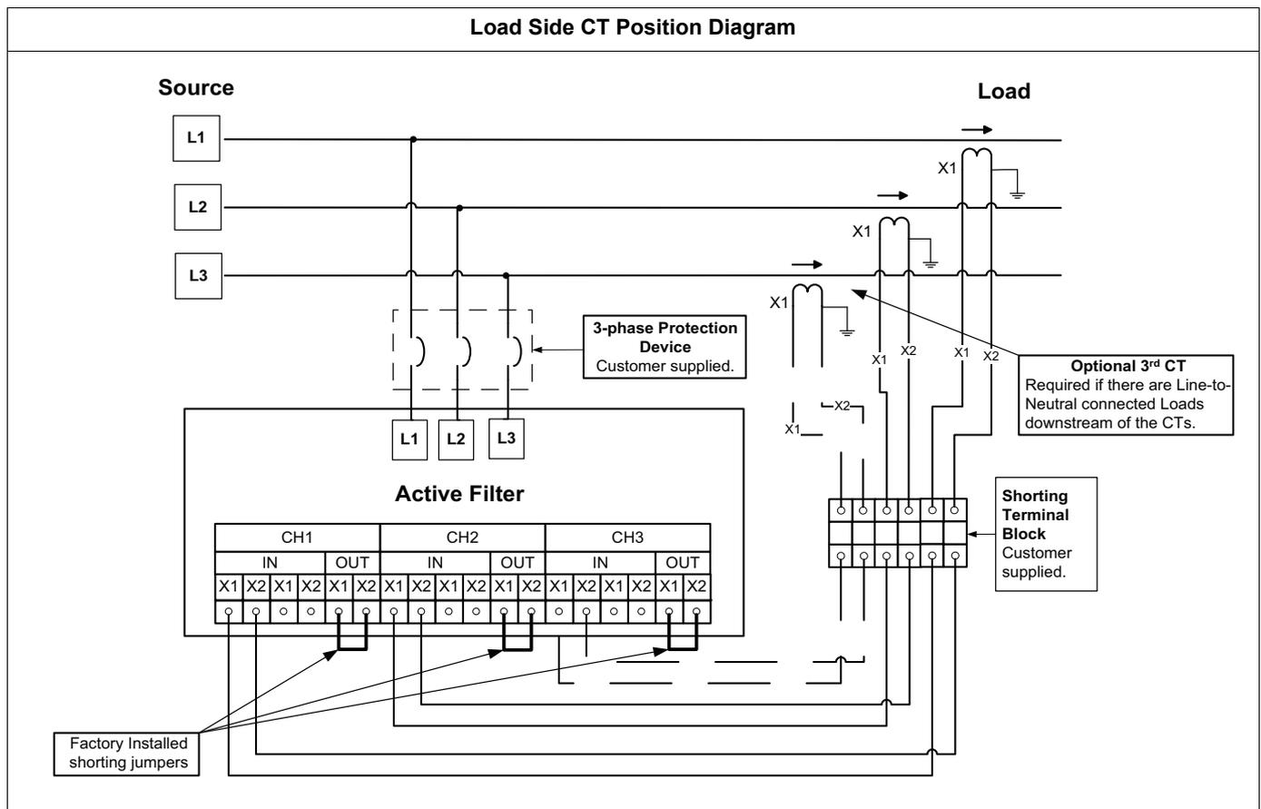
**NOTE:** The factory installed shorting jumpers must be installed.
