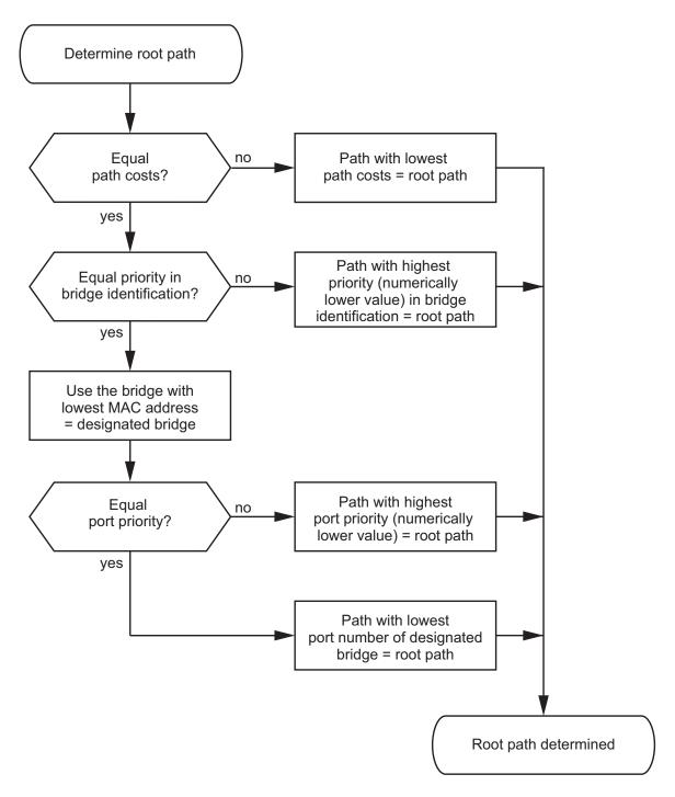
Figure 10: Flow chart for determining the root path
