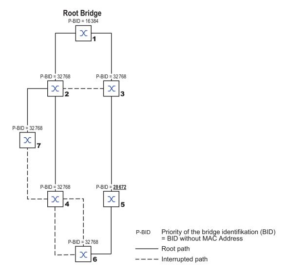
Figure 12: Example of manipulating the root path
