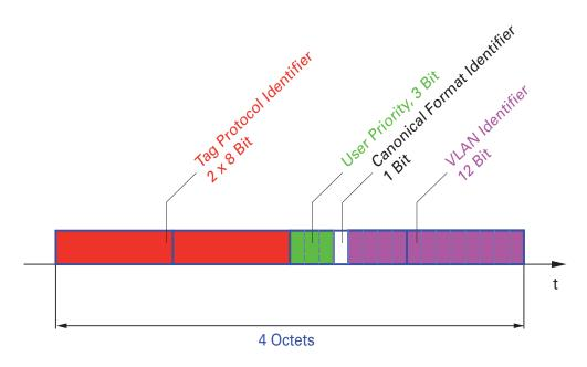
Figure 16: Structure of the VLAN tagging
