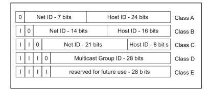
Figure 3: Bit representation of the IP address
