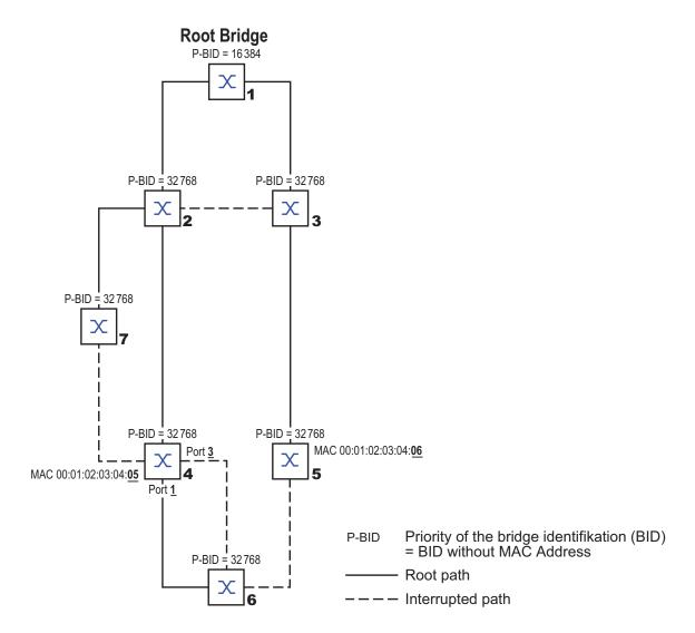
Figure 11: Example of determining the root path
