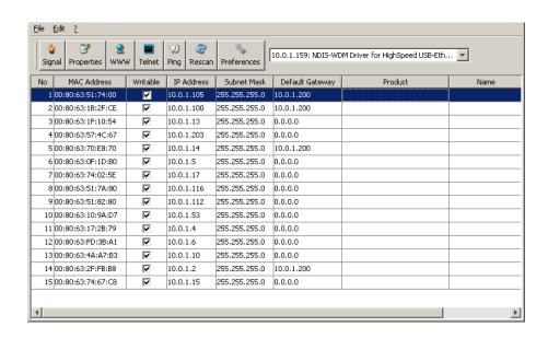
Figure 1: Ethernet Switch Configurator
