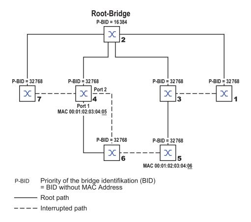
Figure 13: Example of manipulating the tree structure
