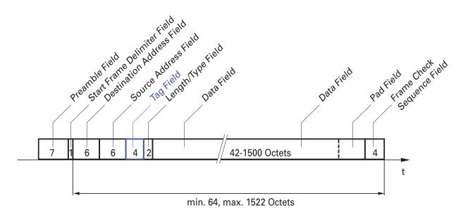
Figure 15: Ethernet data packet with tag
