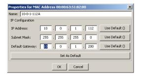
Figure 2: Ethernet Switch Configurator – IP parameter assignment
