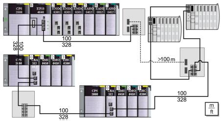
**NOTE:** A BMENOC0301/11 module can support distributed equipment through its Ethernet backplane connection *(see page 80)* to the PAC *and* through the device network port(s) on the front of the BMENOC0301/11, respecting the limitation of 128 scanned devices per BMENOC0301/11 module.
