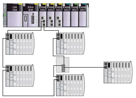
The Ethernet ports on the BMENOC0301/11 module function as both an Ethernet switch and an interface to the module. Information flows through the device to the STB islands in the loop.
