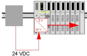
The figure below shows how the 24 VDC signal is distributed to an extension segment across the island:
