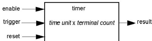
The trigger input starts the timer at 0 and accumulates *time units* of 1, 10, 100 or 1000 ms for a specified number of counts. The reset input causes the timer accumulator to be reset.
