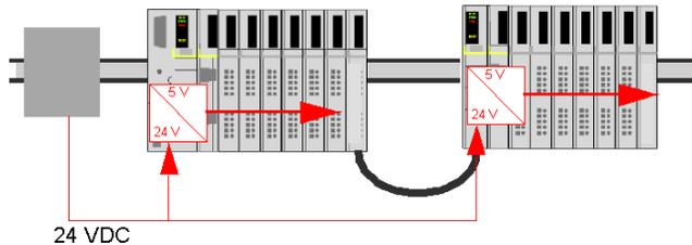
The logic power signal is terminated in the STB XBE 1100 module at the end of the segment (EOS).
