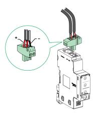
It is recommended to use an UL listed/UL recognized limited voltage/limited current or a class 2 power supply with a 24 Vdc, 3 A maximum.
