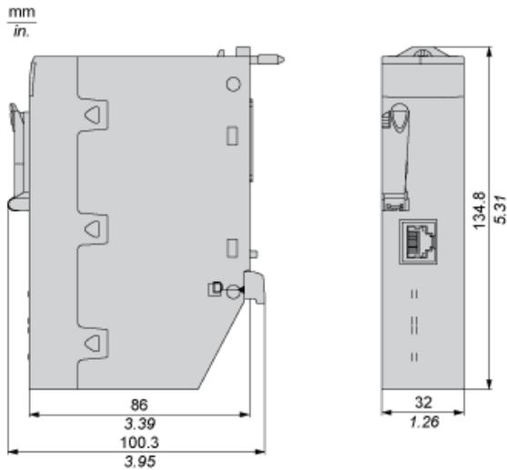
Module Mounted on Rack
