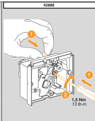
**3** came verrouillage "ouvert" / fitting an open position key lock
