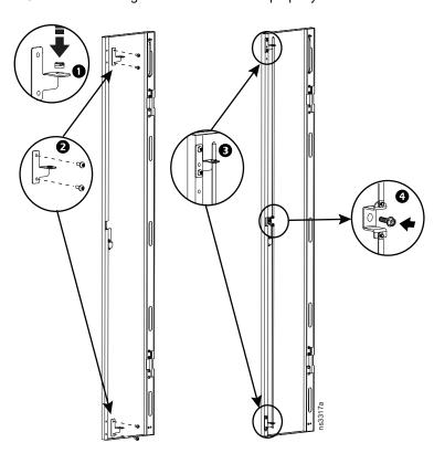
Attach the free end of the ground wires on both doors to the frame using the M6 toothed washers and M6 x 12 pan head T30 screws. The washer is installed between the ground terminal and the cabinet frame. Torque to 28 in-lb (3.2 N-m).
