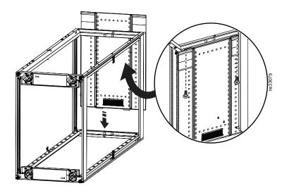
Stand the rack on its casters. Use an open ended 13-mm wrench to lower the leveling feet for support during the remainder of the assembly process
