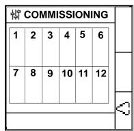
**NOTE:** If you have connected a toroid which is not one of the recommended toroids, then the device should be manually commissioned. See Manual commissioning, page 3. Refer to the Vigilohm catalog for the most up to date listing of compatible toroids.
