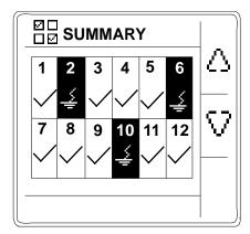
An example of 12 commissioned channel and 3 channels (channel number : 2, 6, and 10) displaying acknowledged insulation alarm is as follows:
