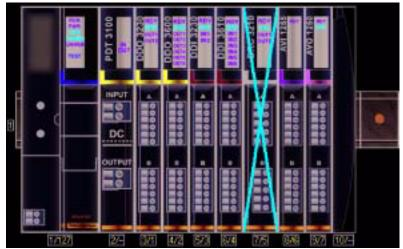
For example, when you physically construct the above configuration, you would build the island without the DRC-3210 and its base.
