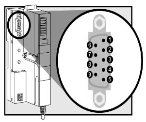
It is recommended that you use a 9-pin SUB-D (DB-9S) connector compliant with DIN 41652 or corresponding international standard. The pin-out should be according to the table below:
