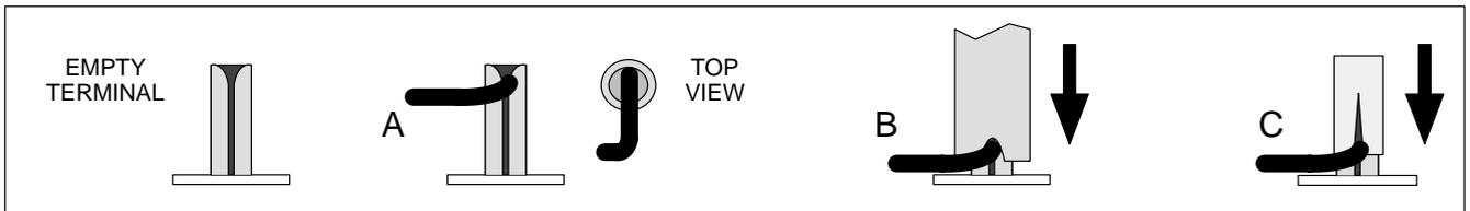
**Figure 7** Wire Terminal Connection (Detail)
