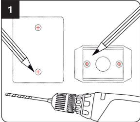
Verify the distance between the KCIN keypad and its remote electronic (refer to page 3 'Notes and Recommendations'). Place the back plate of the KCIN on the wall and the bracket of the remote electronic then mark with a pen the hole location then drill the 2 mounting holes (drill bit Ø 5 mm and 35 MM hole depth) and the hole wiring access.
