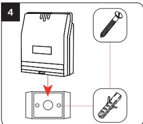
Insert the 2 plastic anchors in the holes. Then mount the bracket of the remote electronics with the M4x30 screws. Slide the box from up to down on the bracket.
