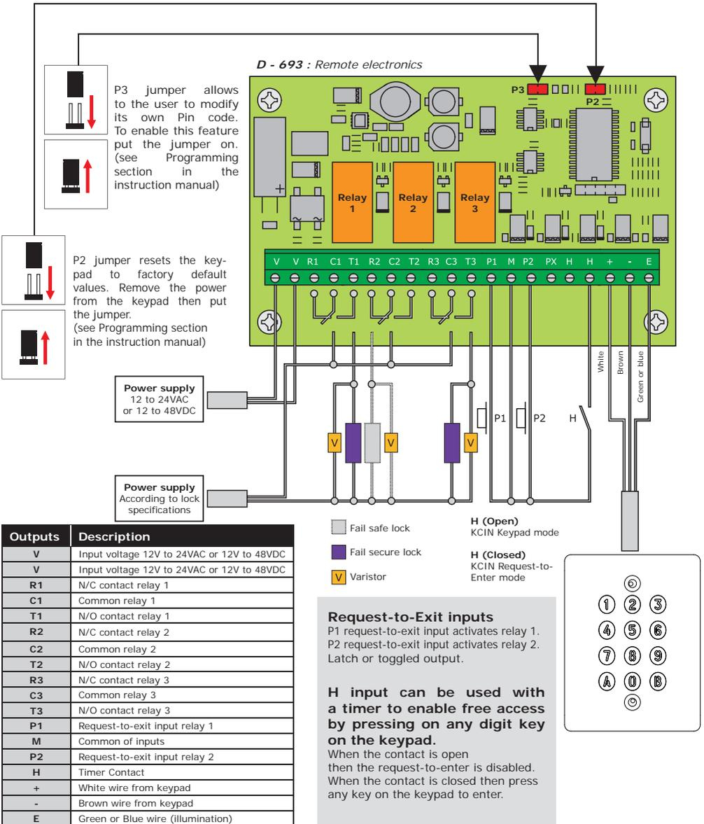
**KCIN****Illuminated weatherproof Keypad with Remote Electronics 1, 2 or 3 relays****Default values**
