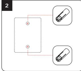
Insert the 2 plastic anchors in the holes. Place the back plate of the KCIN and screw on the wall using the supplied (M4x30) mounting screws.
