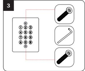
Mount the KCIN keypad on the wall with the M5x35 DIAX® screws.
