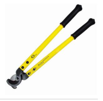
$\sim$  High-grade special tool steel cutting jaws, forged and hardened for an extended working life  $\sim$  Parrotbeak cutting jaws to prevent cable slippage  $\sim$  For large diameter copper and aluminium cables up to 27 mm Ø  $\sim$  Not suitable for steel wire or wire rope  $\sim$  Total length: 530 mm Features & Benefits
