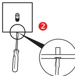
**!** Remove the toggle protection after fitting the finishing plate.
