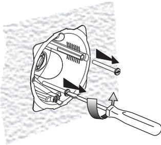
**1** Before installing the mechanism, **remove** the wiring accessory fixing screws from the flush-mounting boxes.
