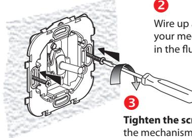
**2** Wire up and then reposition your mechanism in the flush-mounting box.
